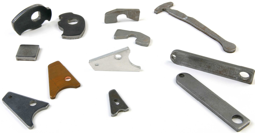
Figure 4: Example of blanked parts from different materials and shapes.
