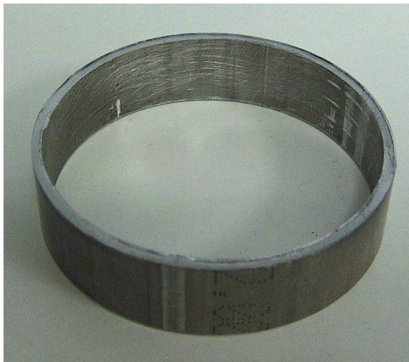
Figure 5b: Cutted steel tube (diameter 60 mm, thickness 2 mm).
